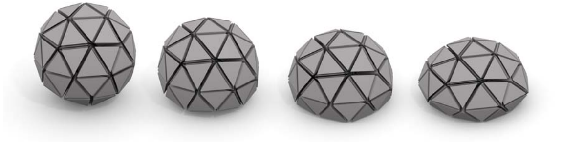
Figure 6.4: (left to right) A spherical s-morph is placed onto a plane and, under gravity, deforms into an ellipsoid. The final stable state occurs when the reaction force from the plane balances against the gravity force.
