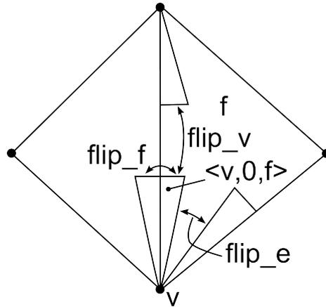
Figure 3: Using a `pos` to navigate a mesh. This figure shows two faces of a mesh and four `pos`'es, drawn as triangles connecting the vertex, edge and face referenced by each `pos`. From the `pos <v,0,f>` (indicated in the figure), we can move to the vertex above it with `flip_v`, the opposing edge within the face with `flip_e`, or to the adjacent face with `flip_f`. If the mesh is fully connected we can reach any position on the mesh using a sequence of these operations.
